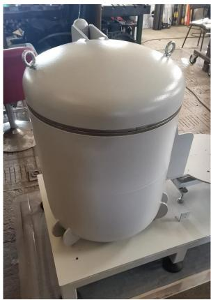
All shields feature an annular lead back shield compatible with remote detector chamber (RDC)
